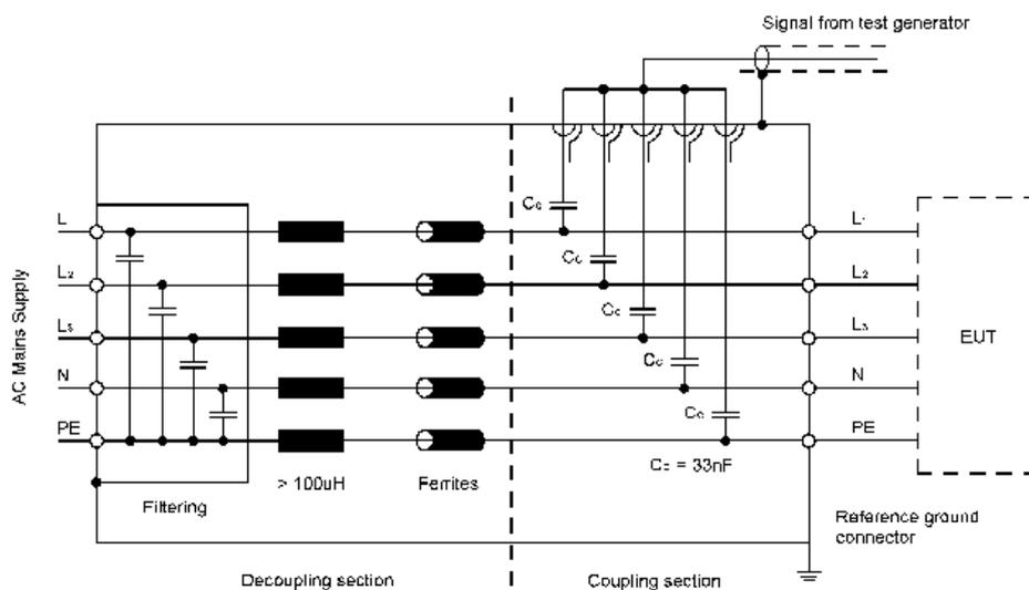
**Figure 4-Coupling/decoupling network for a.c./d.c. power mains supply ports/terminals**
