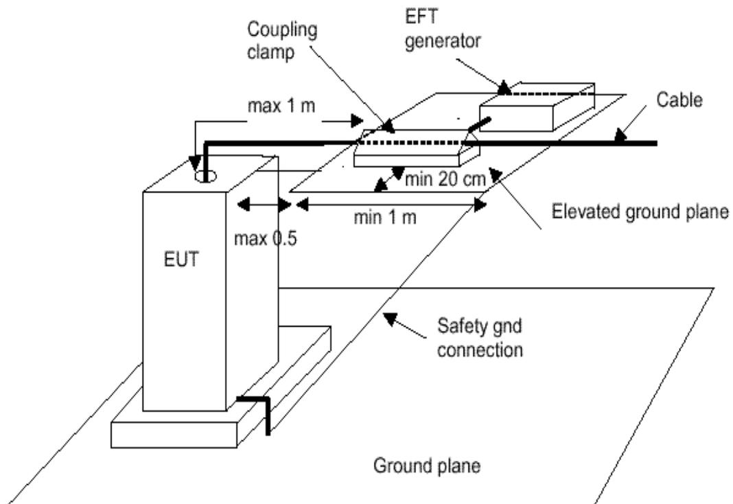
**Figure 7b-Example of a test set up for rack mounted equipment**
