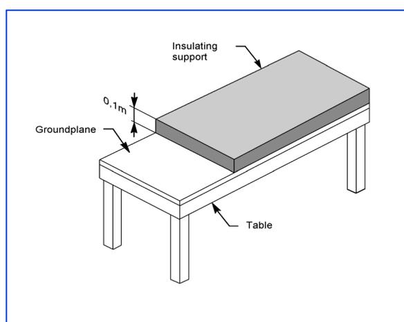
**Figure 7a – Test set-up for table-top equipment**
